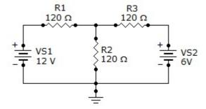
3-b. Find the resistance R1 in Figure ,to transfer maximum power to R2 . (CO1)
