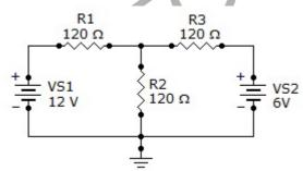
3-b. Find the resistance R1 in Figure ,to transfer maximum power to R2 . (CO1)
